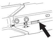
• Tighten both of the screws holding the cutting head using a T-wrench.
